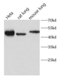
Various lysates were subjected to SDS PAGE followed by western blot with FNab10420(CAV1 antibody) at dilution of 1:1000
