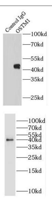
IP Result of anti-OSTM1 (IP:FNab06036, 4ug; Detection:FNab06036 1:500) with mouse brain tissue lysate 4000ug.
