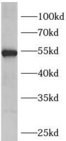
K-562 cells were subjected to SDS PAGE followed by western blot with FNab03265(FZR1 antibody) at dilution of 1:1000
